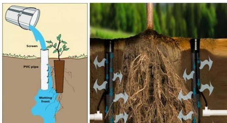
Fig. 5. Deep pipe irrigation system
